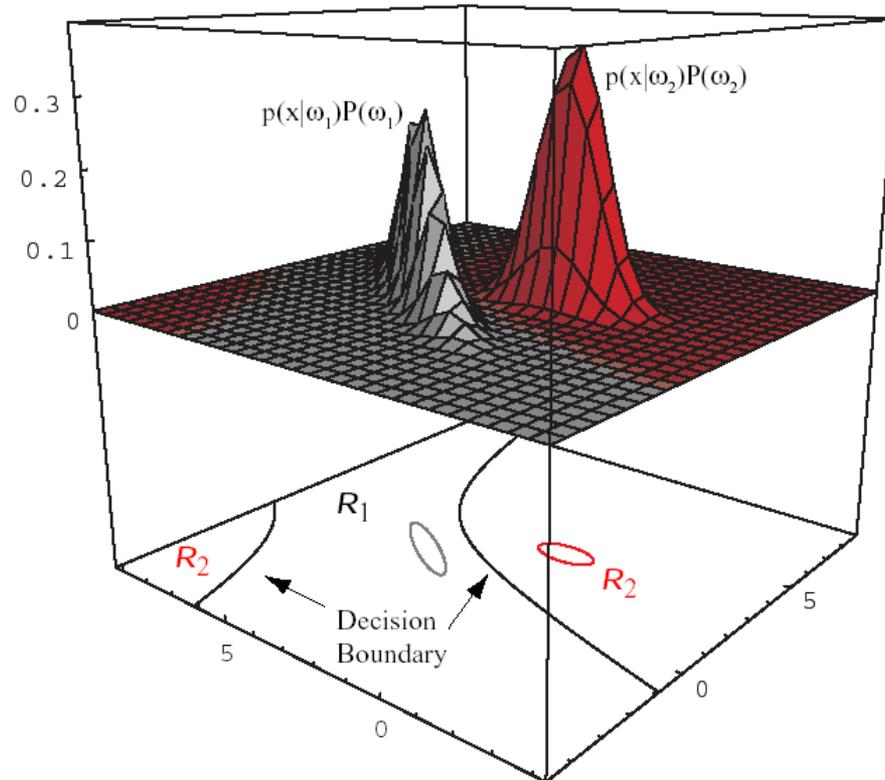
$$g_i(\mathbf{x}) = -\frac{1}{2}(\mathbf{x} - \boldsymbol{\mu}_i)^t \boldsymbol{\Sigma}_i^{-1} (\mathbf{x} - \boldsymbol{\mu}_i) - \frac{d}{2} \ln 2\pi - \frac{1}{2} \ln |\boldsymbol{\Sigma}_i| + \ln P(\omega_i).$$
