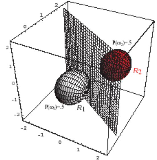
$$g_i(\mathbf{x}) = -\frac{1}{2}(\mathbf{x} - \boldsymbol{\mu}_i)^t \boldsymbol{\Sigma}^{-1}(\mathbf{x} - \boldsymbol{\mu}_i) + \ln P(\omega_i)$$
