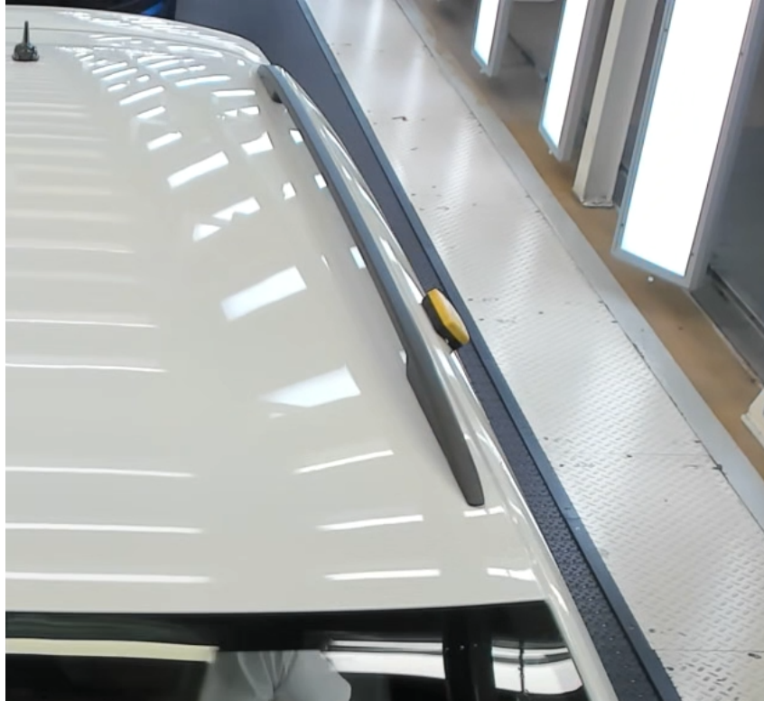
Figure 1.1: RFID (Radio Frequency Identification) module (yellow box) attached to the roof of every vehicle is used to provide the car maker with exact localization of the car.
