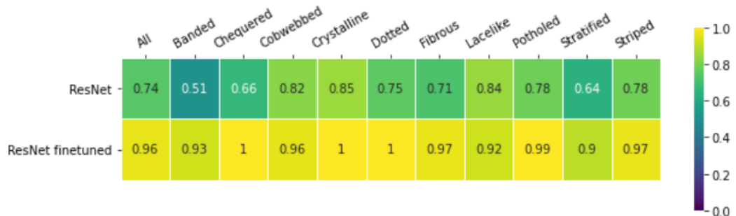
Figure 6.11: Comparison of mAP of ResNet152 and fine-tuned ResNet152 on different categories on Patterns dataset.
