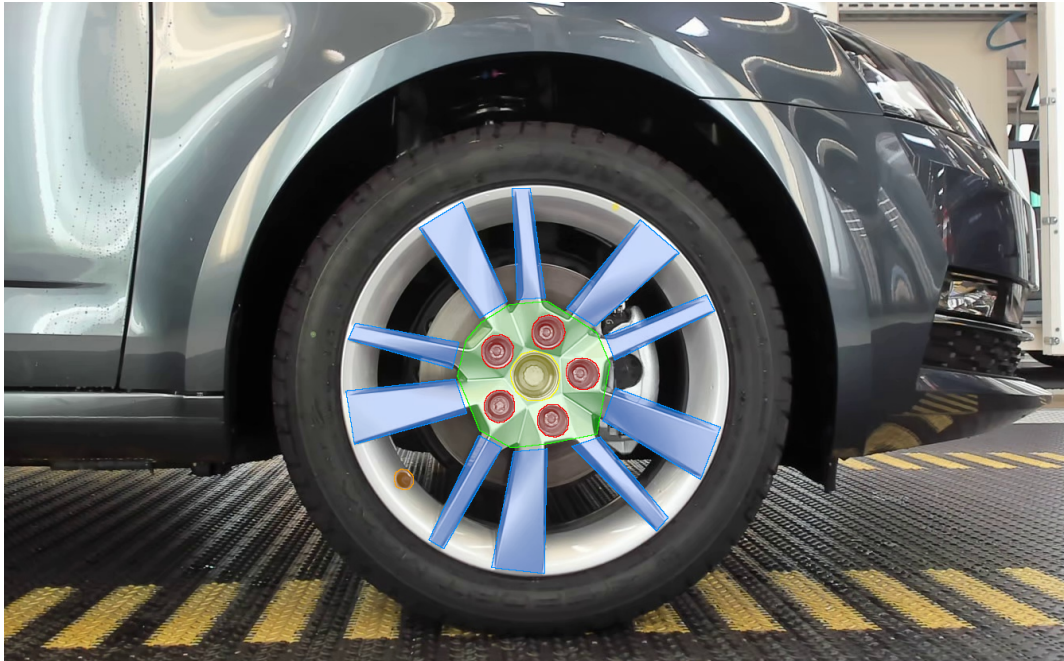
Figure 1.2: Rim structure - center hole is marked yellow, center disc is green, spokes are blue, valve stem is orange and bolt holes are red.
