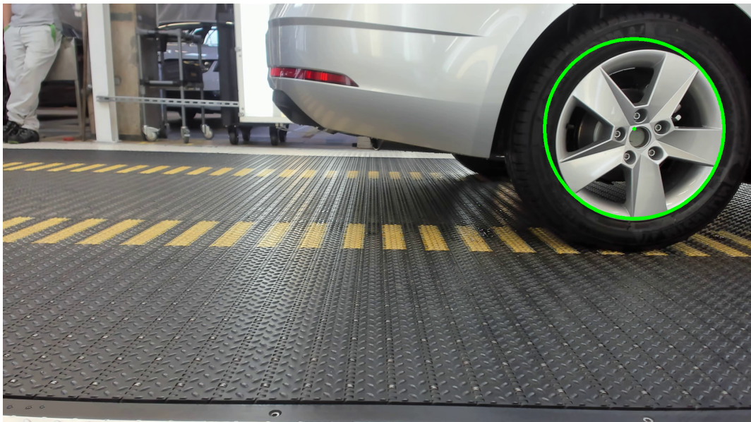
Figure 4.2: Frame showing elliptical shape of the rim near the edge of the frame - the green circle is detection of the rim by Hough transform for circles.
