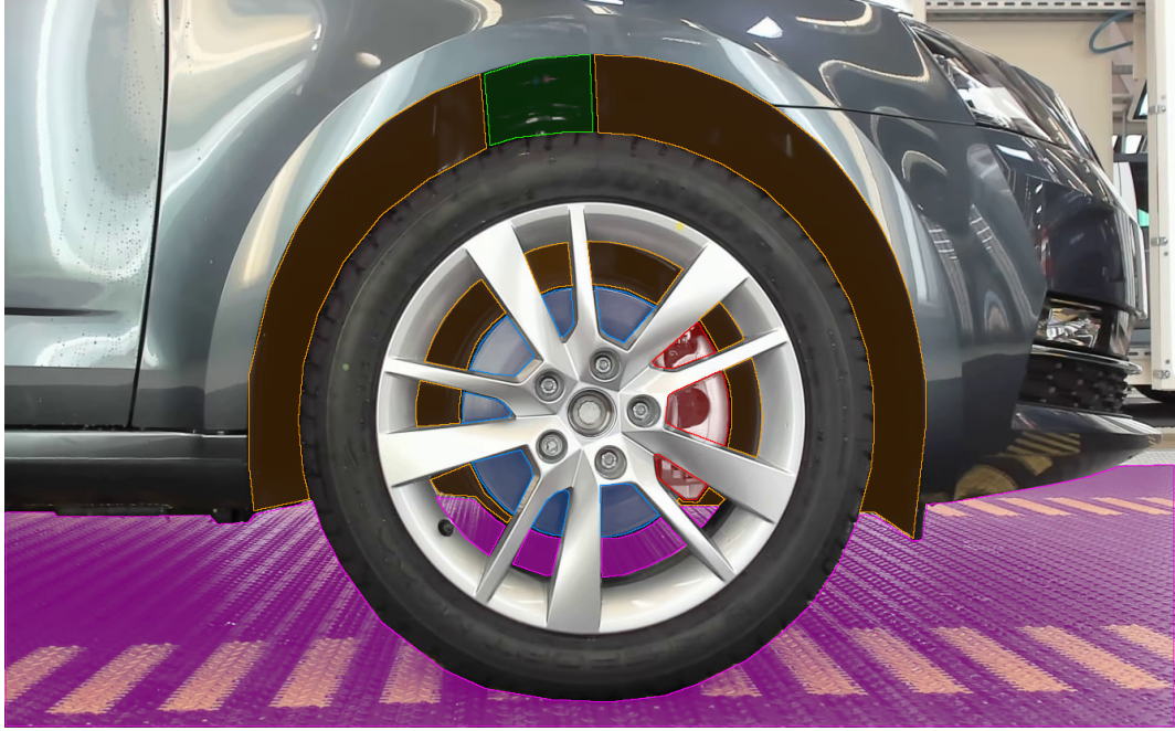
Figure 1.4: Nearby Components - brake disc is marked blue, brake is red, suspension system is green, other space visible inside a car is orange and conveyor belt is violet.
