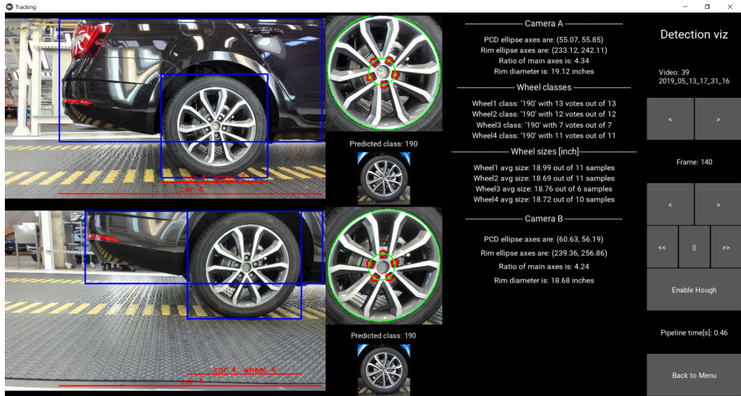
Figure 5.3: User interface of the prototype - on the left side there is Frame_a and Frame_b, next to them are visualizations of ellipse estimations and predicted classes. The texts under heading 'Camera A/B' sum up information about size estimation for the current frame. The texts under headings 'Wheel classes/sizes' sum up aggregated knowledge we have about the classes and sizes of the rims on the currently tracked car.
