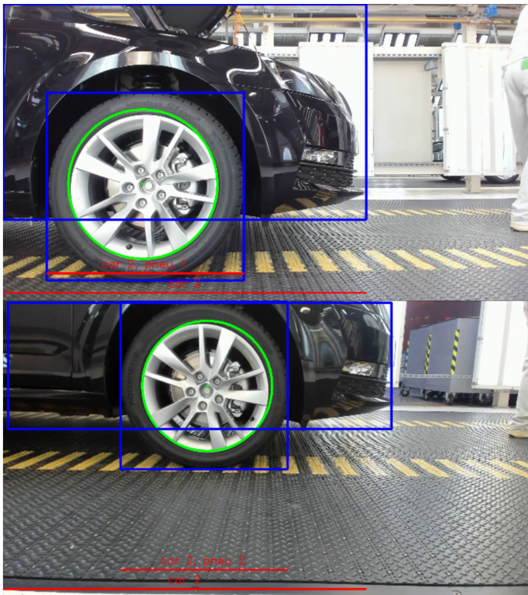
Figure 5.1: Custom tracking algorithm - see difference in position and size of a car and its wheel. The camera A in the top and camera B in the bottom.
