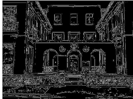
low threshold (weak edges)
